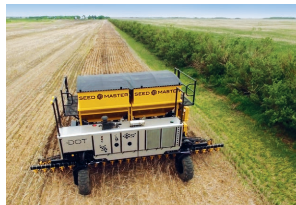
Made in Saskatchewan: DOT Power Platform is an autonomous system for powering implements.
